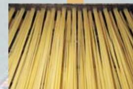
To prevent the pasta from sticking together in the drying process, long pasta is subject to a blast of air immediately after extrusion. Short pasta is transferred to a shaking pre-dryer to ensure it is separated.
